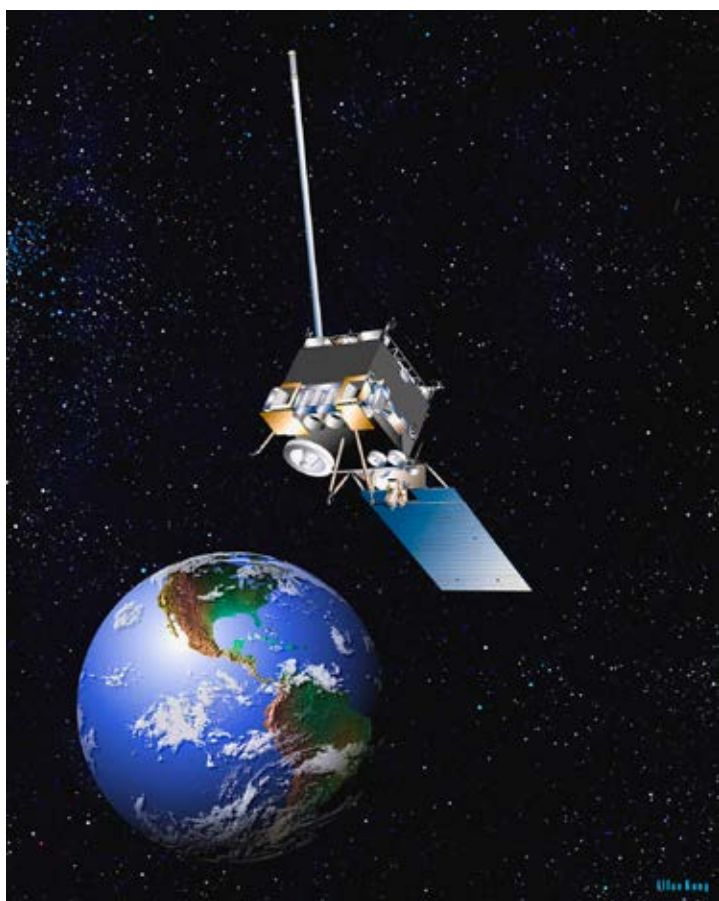
NOAA’s geostationary operational environmental satellite, or GOES, tracks heat waves by detecting cloud-free areas of the atmosphere that heat up quickly Credit: NOAA
